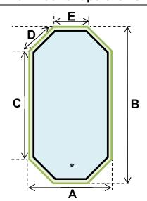
Measure from line to line, which should extend 12" beyond each corner of your pool, to determine the **Cover Size**.
